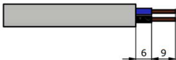
Correct placement strain relief cap
